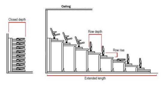
\* Note that there should be a minimum of 2.1m between the top deck and the ceiling of the room.
